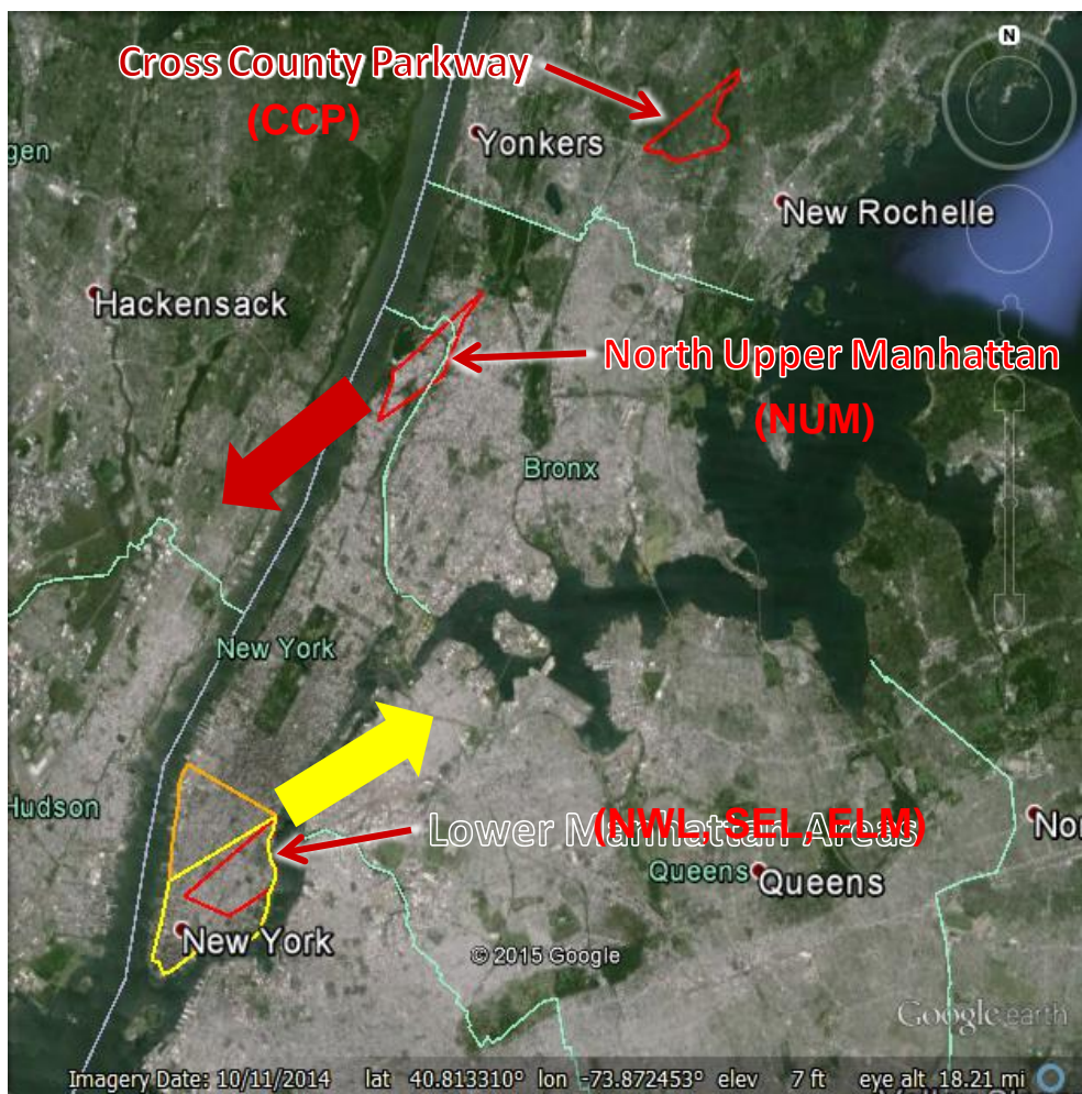
Figure 3. Areas with sufficient methane survey data to support experimental application of simple mass balance emissions estimate method. Bold yellow and red arrows indicate predominant wind direction on days for which there was available methane survey data for areas marked with the same colors (yellow or red). There were 3 areas in Lower Manhattan (see Figure 4).
