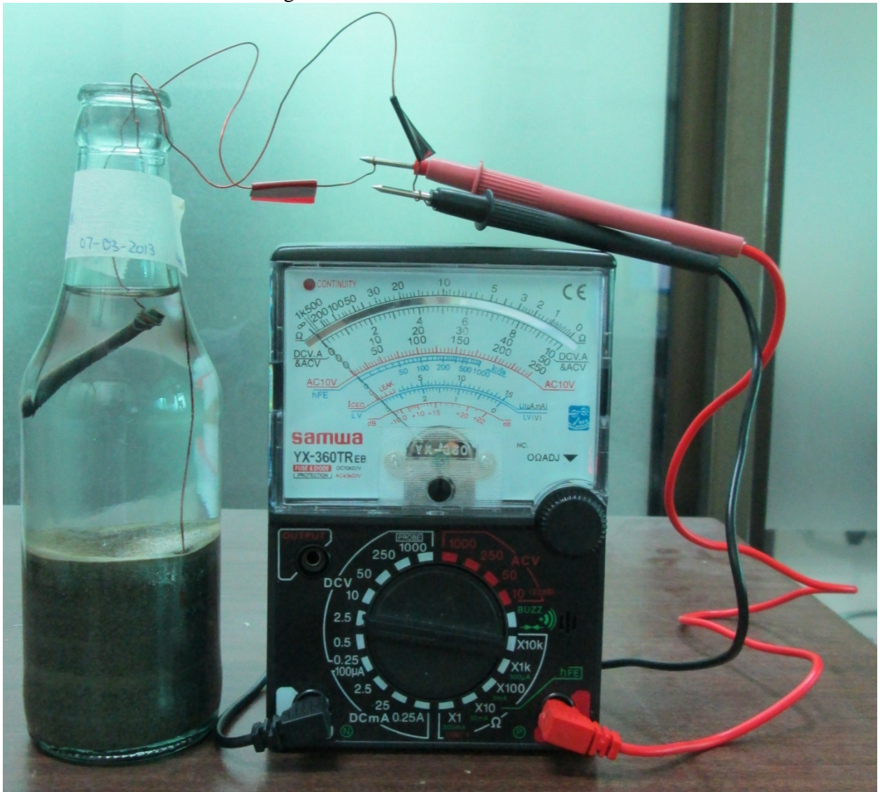
Fig. 2. Lab scale MFC Construction
