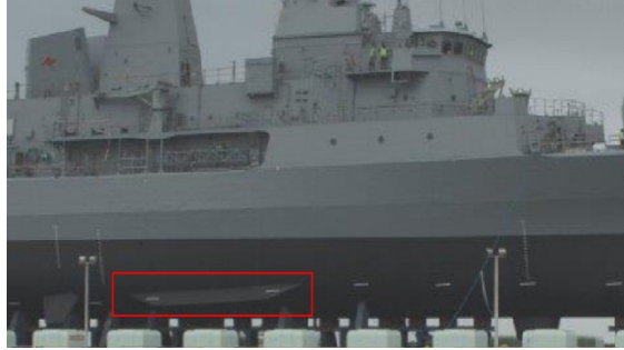
Figure 10 - Example of Bilge Keel on RAN ANZAC Frigate
