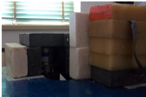
Fig. 2. Experimental set up for semiconductor gamma detector and isotopic neutron source. On the right, the Am-Be source contained in its paraffin moderator. On the left, the Ge(Li) detector surrounded by lead shielding.
