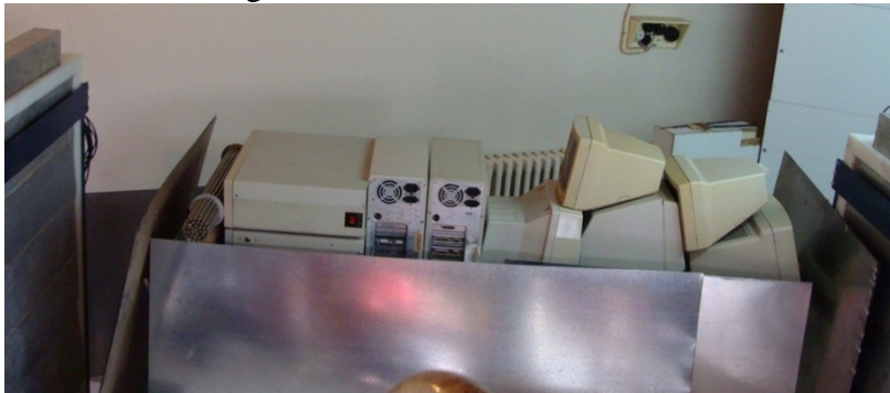
Fig. 1. Experimental simulated cargo array irradiated with an accelerator neutron source. The neutron beam impinges from the right. The neutron panel detectors appear in each side of the image and on the left, a natural uranium fuel element is visible.
