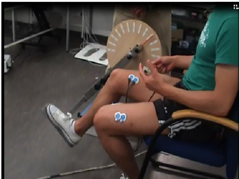
Figure 2. Measuring electrical activity of the muscles in different angles of knee extension
