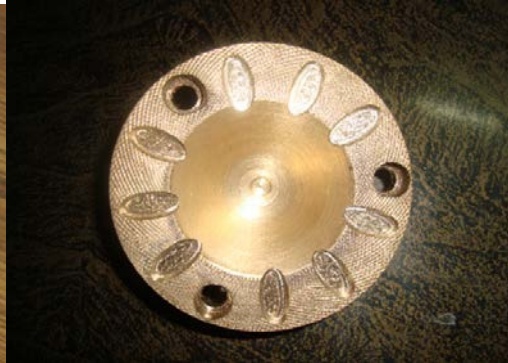
Figure: 5 Photo Graphic View of Brass Crown Piston with 9 grooves (BP9)
