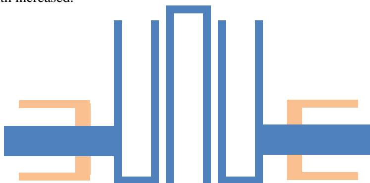
Figure 10: Layout of three poles hairpin line BPF with defected ground structure
