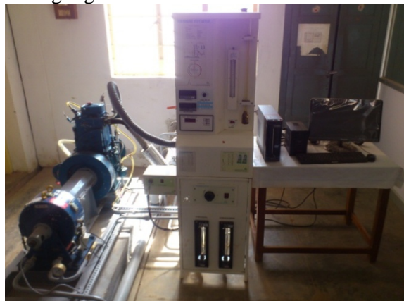
Figure3. Experimental set up of Insulated Engine Test Rig
