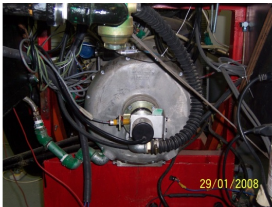
Figure 11: Rotary encoder (Crank Angle) Sensor and Dynamometer
