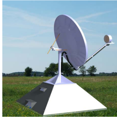
Figure 3. Parabolic concentrator design with in focus heater
