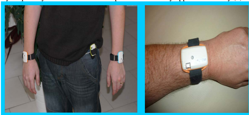
Picture 1, 2 Appearance of sensor – accelerometer
