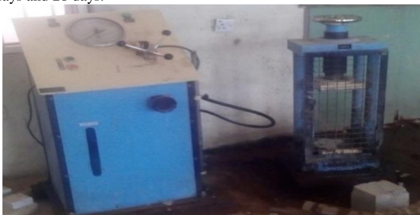
Plate 4: Manual and automatic compressive testing machines
