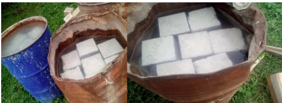
Plate 3: Concrete cubes immersed in water in a curing tank
