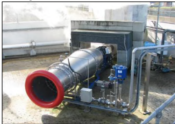
Fig. 16 the pre-cooler will be tested at RELS B9 Test site using a VIPER 522 jet engine
