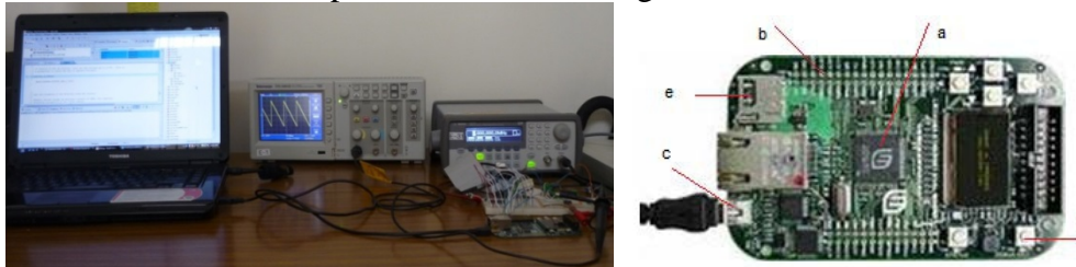
Figure 6. User interface, Prototype board, Signal viewer. Development board: The LM3S6965 prototyping a) ARM® Cortex-M3 Processor, b) GPIO, c) USB port, d) Reset, e) Memory card slot for data and/or program.
